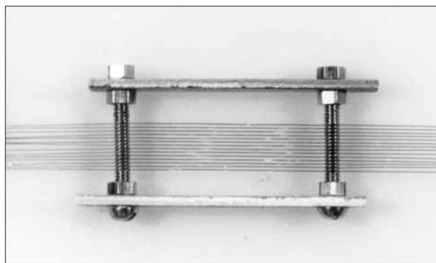
Fig. 1. The 2003 wire diffraction grating using brass bolts with 80 threads per inch.
